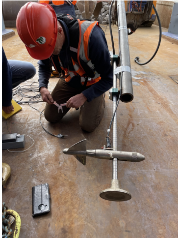
(a) OTT-meter mounted to crane
