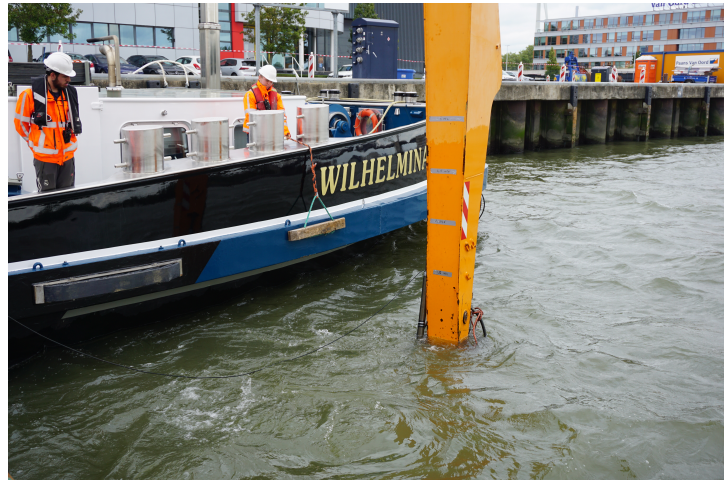
(b) Free flow measurement with the OTT-meter mounted to a crane
