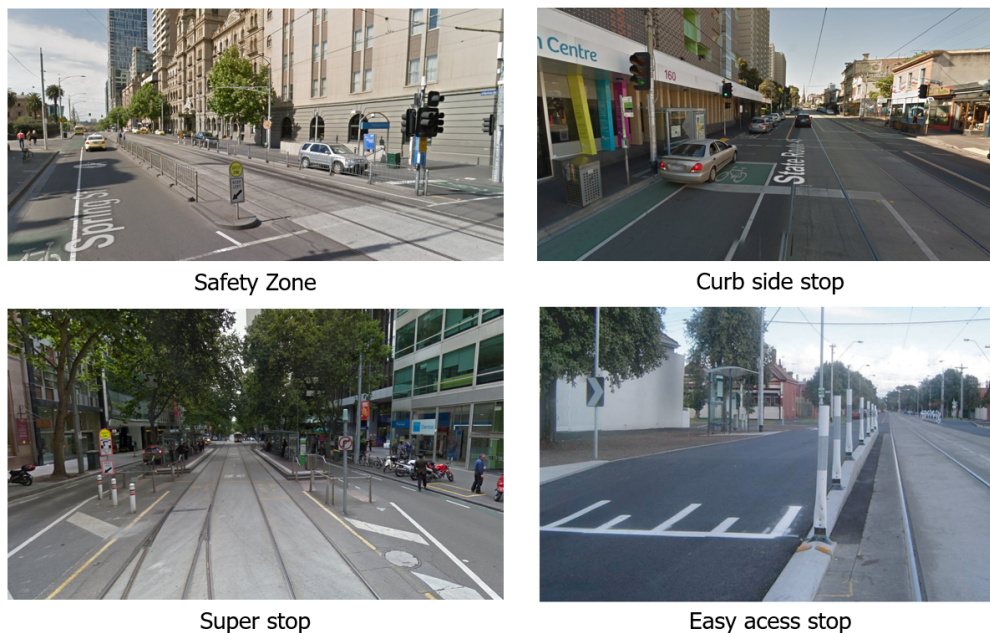
Figure 2.3: Tram stop designs in Melbourne, Australia Source: Currie and Smith, (2006) ; Currie and Reynolds, (2010) ; Google Earth StreetView; Own Elaboration (2019)
