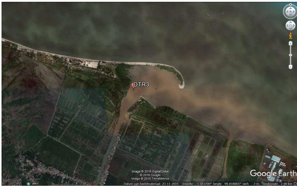
Figure 30 Google Earth Image 2015 showing spit forming indicating a net eastward directed sediment transport
