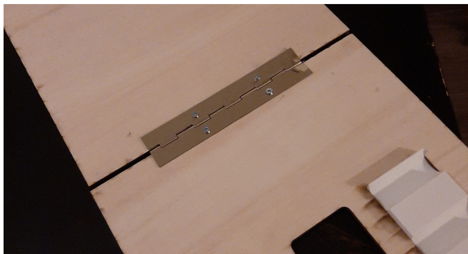
Figure 60 180-90 deg hinge in the mattress board
