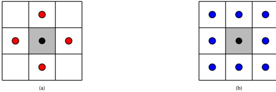
Figure 6.3: (a) Compact face-based stencil on the example of a structured quadrilateral mesh. (b) Extended node-based stencil on the example of a quadrilateral triangular mesh.
