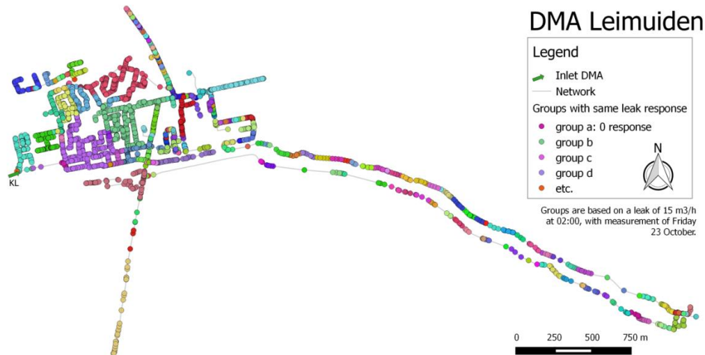
Figure I.1 Result groups with a leak of 15 \text{ m}^3/\text{h} during minimum flow. Groups when the sensor placement optimization with a leak of 7.5 \text{ m}^3/\text{h} during minimum flow is used.
