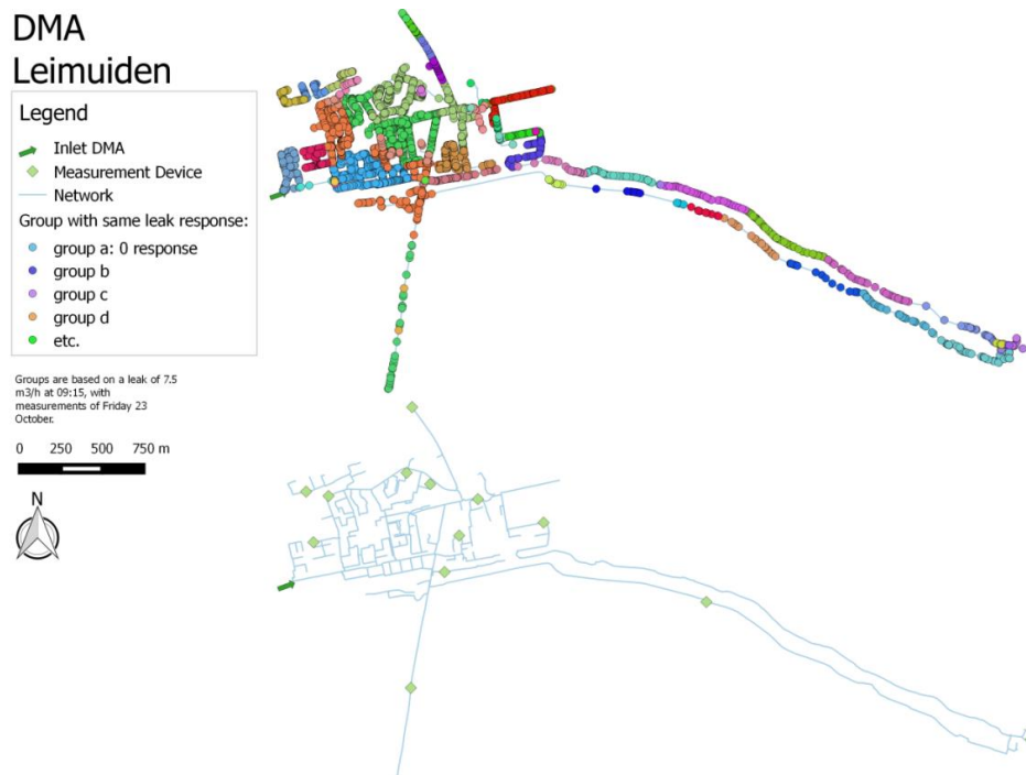
Figure I.2 Result sensor placement optimization with a leak of 7.5 \text{ m}^3/\text{h} during maximum flow. Top: groups with nodes that have the same leak response. Bottom: proposed location of measurement devices.
