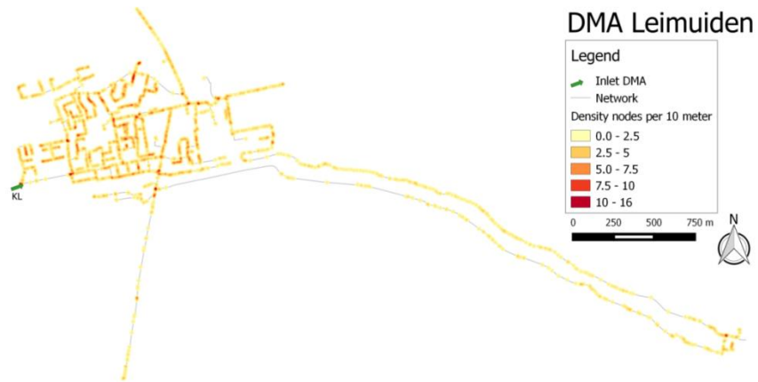
Figure E.1 Node density heat map. Darker colors indicate a higher density of nodes.
