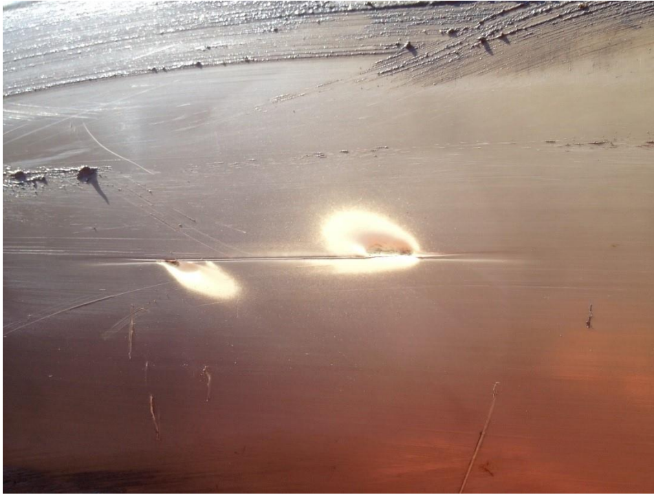
Figure A.1 Example of enlarged leak due to moving ground particles
