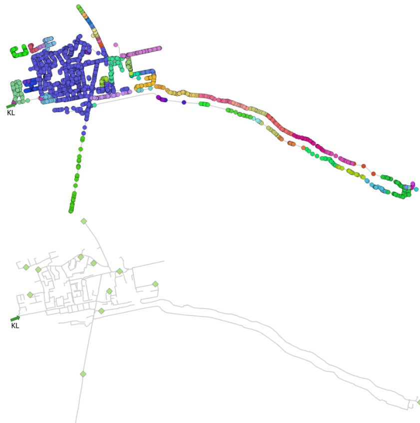
Figure 3.1 Result sensor placement optimization with a leak of 7.5 \text{ m}^3/\text{h} during minimum flow. Top: groups with nodes that have the same leak response. Bottom: proposed location of measurement devices.
