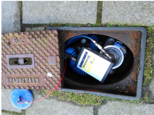
Figure 2.2 Pressure logger attached to a fire hydrant
