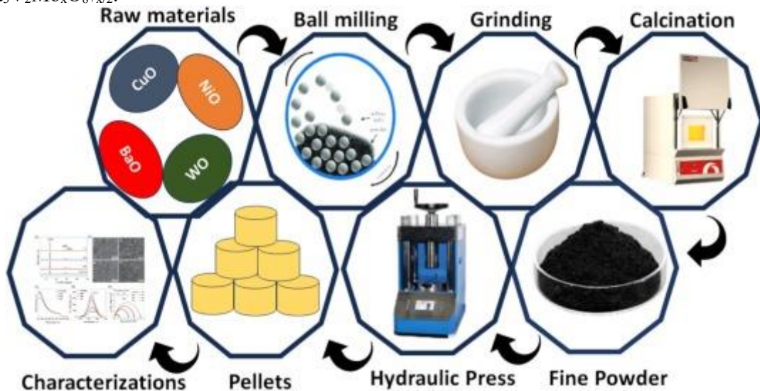
Figure 5. Process of Solid-State Reaction for Perovskite Materials [66].
