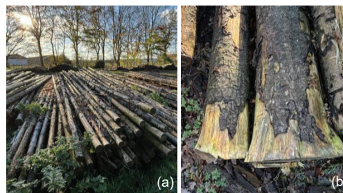
Figure 1. (a) timber piles after cutting; (b) typical deviation of the bottom part of a tree trunk.
