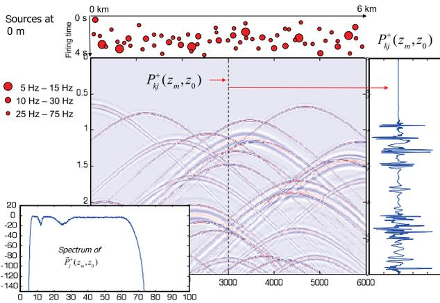
Figure 4. Incident wavefield at  $z_m = 1000$  m, generated by a DSA at  $z_0$  with three narrowband source units at 10, 20, and 50 Hz, together with its amplitude spectrum, the Fourier transformation being applied to the laterally averaged autocorrelation function. Note that the incident wavefield at gridpoint  $i$ ,  $p_{ij}^+(z_m, z_0)$ , represents a dispersed time series.
