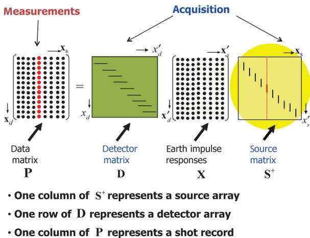
Figure 1. The data matrix represents a frequency slice of the total seismic data volume, the complex-valued scalar of each matrix element representing one Fourier component of a seismic trace. The model of the data matrix ( $\mathbf{P}$ ) consists of the source matrix ( $\mathbf{S}^+$ ), the earth's transfer matrix  $\mathbf{X}$  and the detector matrix  $\mathbf{D}$ .
