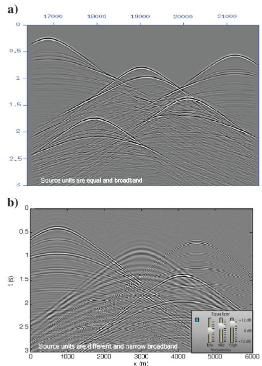
Figure 3. (a) A blended shot record that is generated by five equal broadband source units and five different narrowband source units, representing homogeneous and inhomogeneous blending, respectively. Note that with inhomogeneous blending frequency shaping becomes an option in the field for the compensation of absorption.
