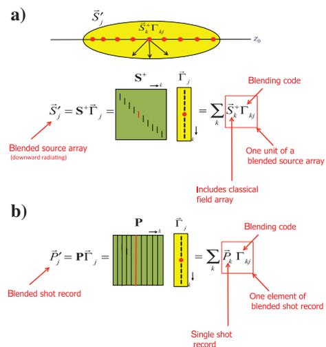
Figure 2. (a) One blended source array consists of a multitude of source units, each unit having its own code; (b) a blended shot record can be written as a linear combination of single shot records that are generated by the individual source units of the blended source array.
