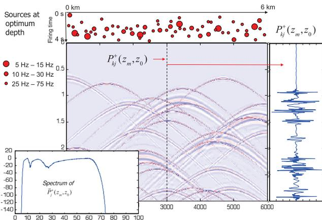
Figure 6. The same experiment as in Figure 5, but now for a variable depth level for each source unit, choosing  $z_k = 0.25c_w/f_c$  (ghost matching).
