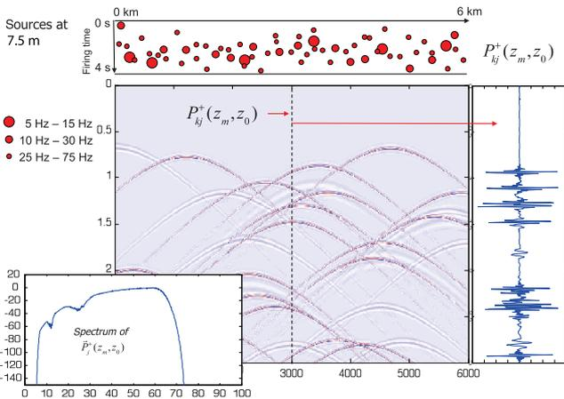
Figure 5. The same experiment as in Figure 4, but now for the marine situation, using a fixed depth level of 7.5 m for all source units.
