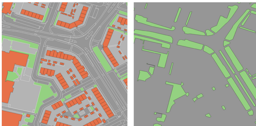
Fig. 12. Left: original BGT data; Right: after conversion into hard/soft values and aggregation.
