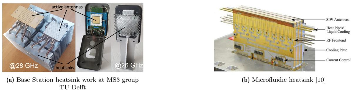
**Figure 1.1:** Examples of heat management structures
