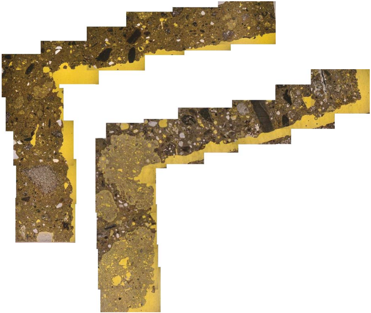
Fig. 19. Microphotographs over the bend in a tooled Ettringen (above) and Weibern (below) tuff mullions. Note the absence of any microcracks.
