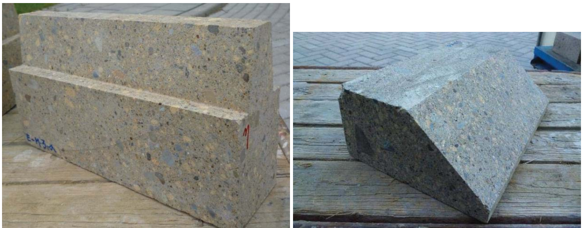
Fig. 3. Examples of cut mullion and window sill.
