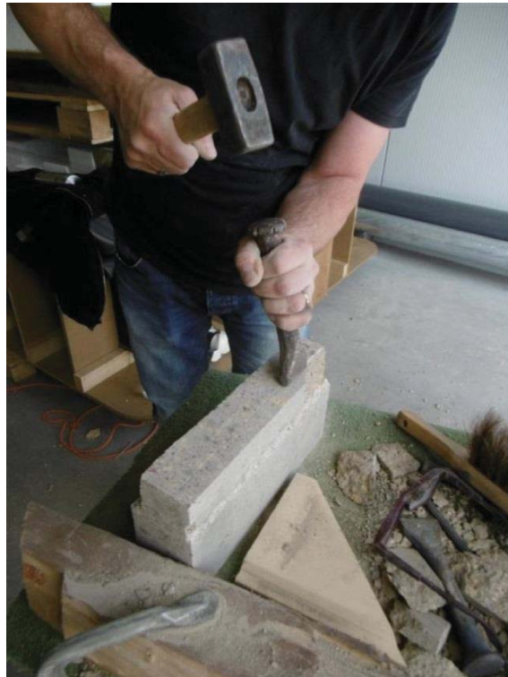
Fig. 4. Making of a mullion by hand.
