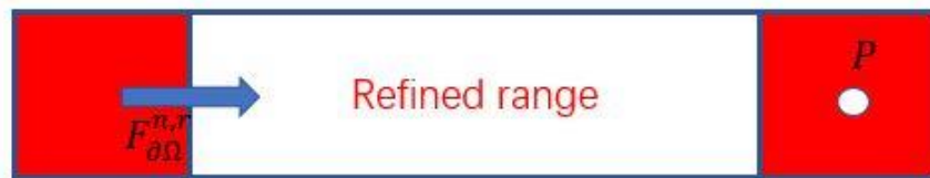
Figure 3.10. Refined zone mathematics model including Neumann boundary condition and Dirichlet boundary condition
