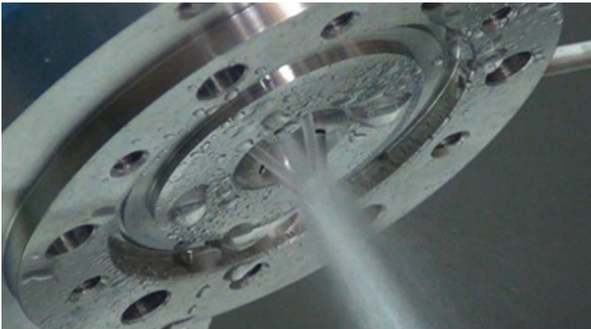
Figure 4.24: Cold-flow test of impinging jet injector showing atomisation [51]
