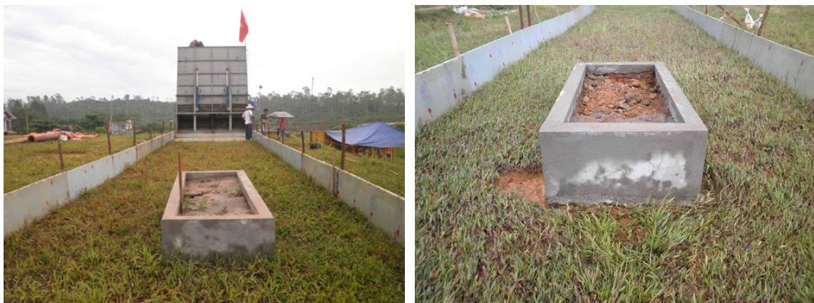
Figure 6.9: Grass mat around the square obstacle at YB4. Left: initial condition. Right: after 40x2 + 60x6.
