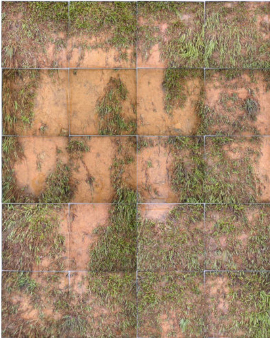
Figure B.39: 60x4 + 80x6 + 100x10, 30 to 34 m from the dike crest, section YB3.
