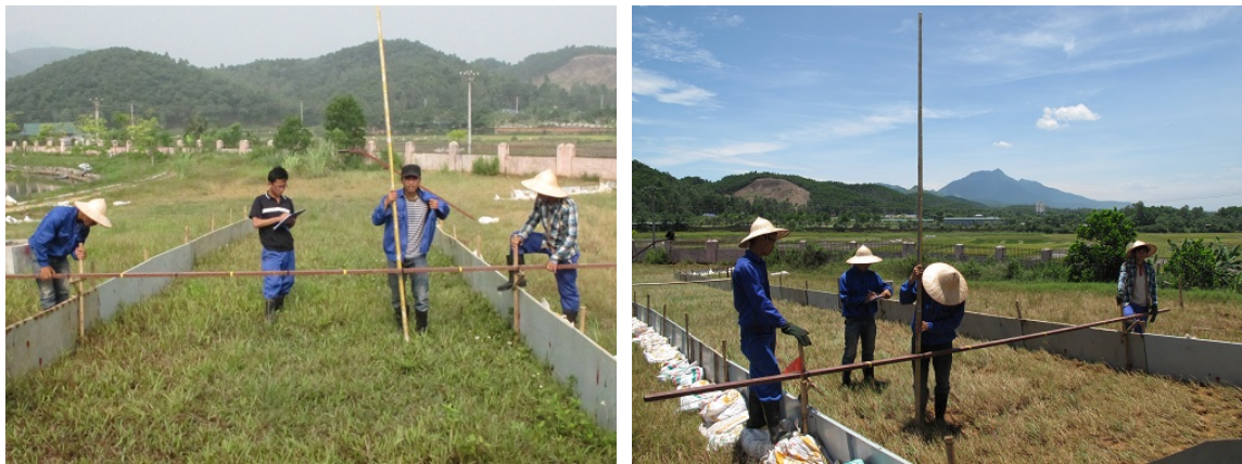
Figure 4.1: Measurement of the dike slope profile.
