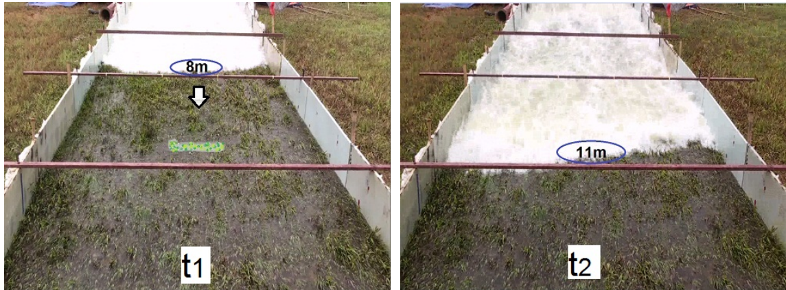
Figure 3.3: A series of two images in which the front part of overtopping flow traveled over a distance of 3 m within \Delta t seconds.
