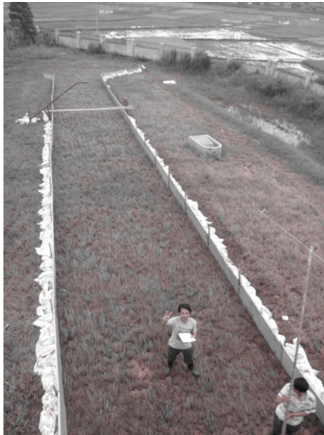
Figure 2.9: Section YB2, plain slope covered by Bermuda grass.
