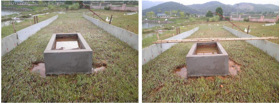
Figure 6.10: Damage around the square obstacle at YB4. Left: after 0 \times 2 + 60 \times 6 + 80 \times 4 . Right: after that 80 \times 2 + 100 \times 4 .
