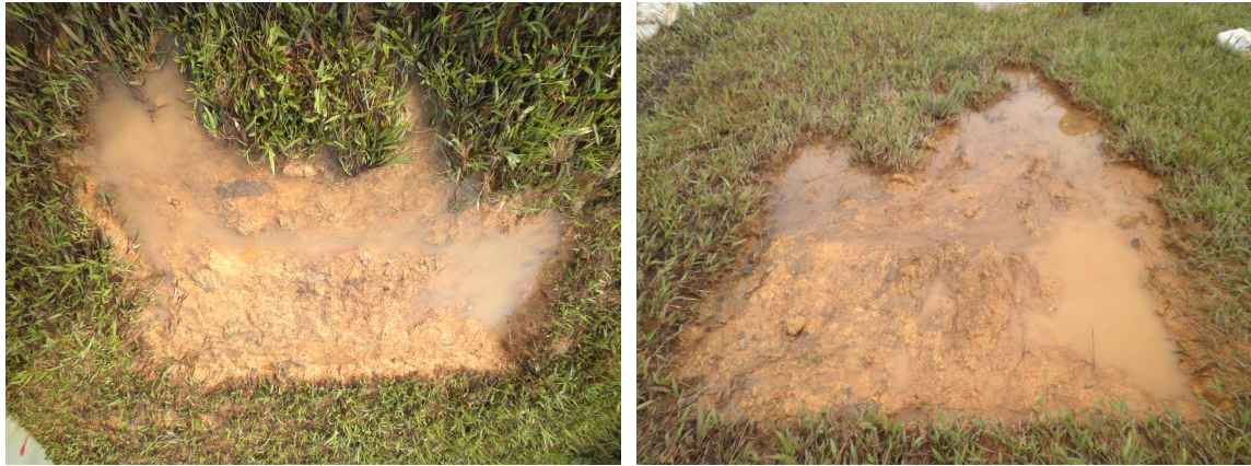
Figure 6.12: The 5bc damage after 40x1 + 60x2 (left) and after that 60x4 + 80x6 + 100x6 (right), wave height of 2.0 m.
