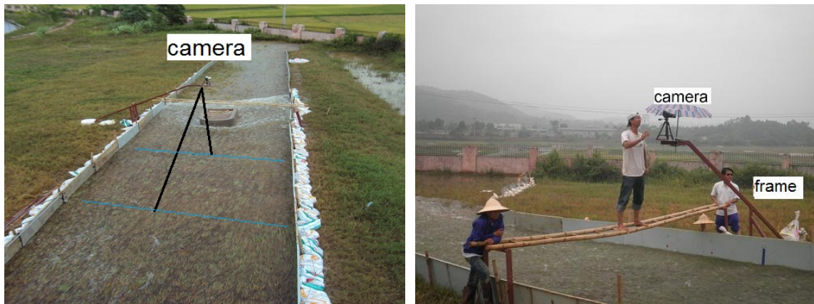
Figure 3.1: Set-up of the camcorder to capture overtopping flow on the dike slope
