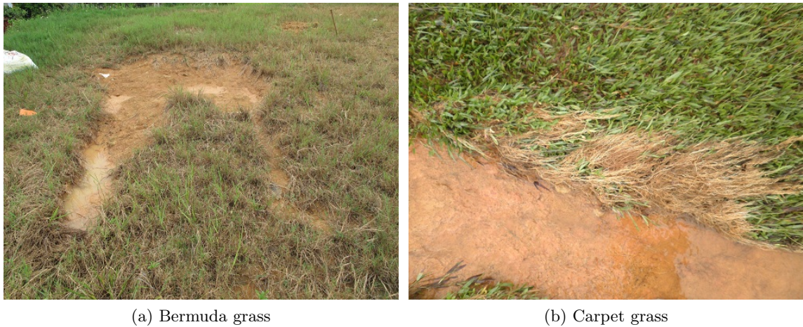
Figure 6.13: Mechanism 'roll up' on slopes covered with Bermuda and Carpet grass.
