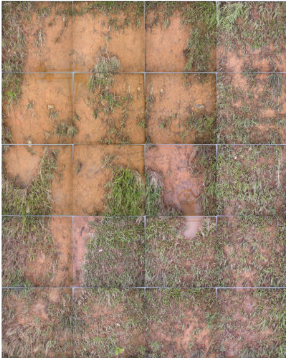
Figure B.43: (60x4 + 80x6 + 100x10) with H_s = 1.5 m and (40x1 + 60x2 + 80x2 + 100x1) with H_s = 2.0 m, 30 to 34 m from the dike crest, section YB3.
