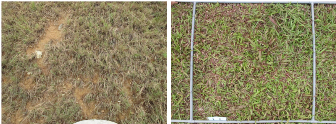
Figure 2.7: Two local grass species protect the 1/15 slope, Bermuda grass (left) and Mat grass (right).
