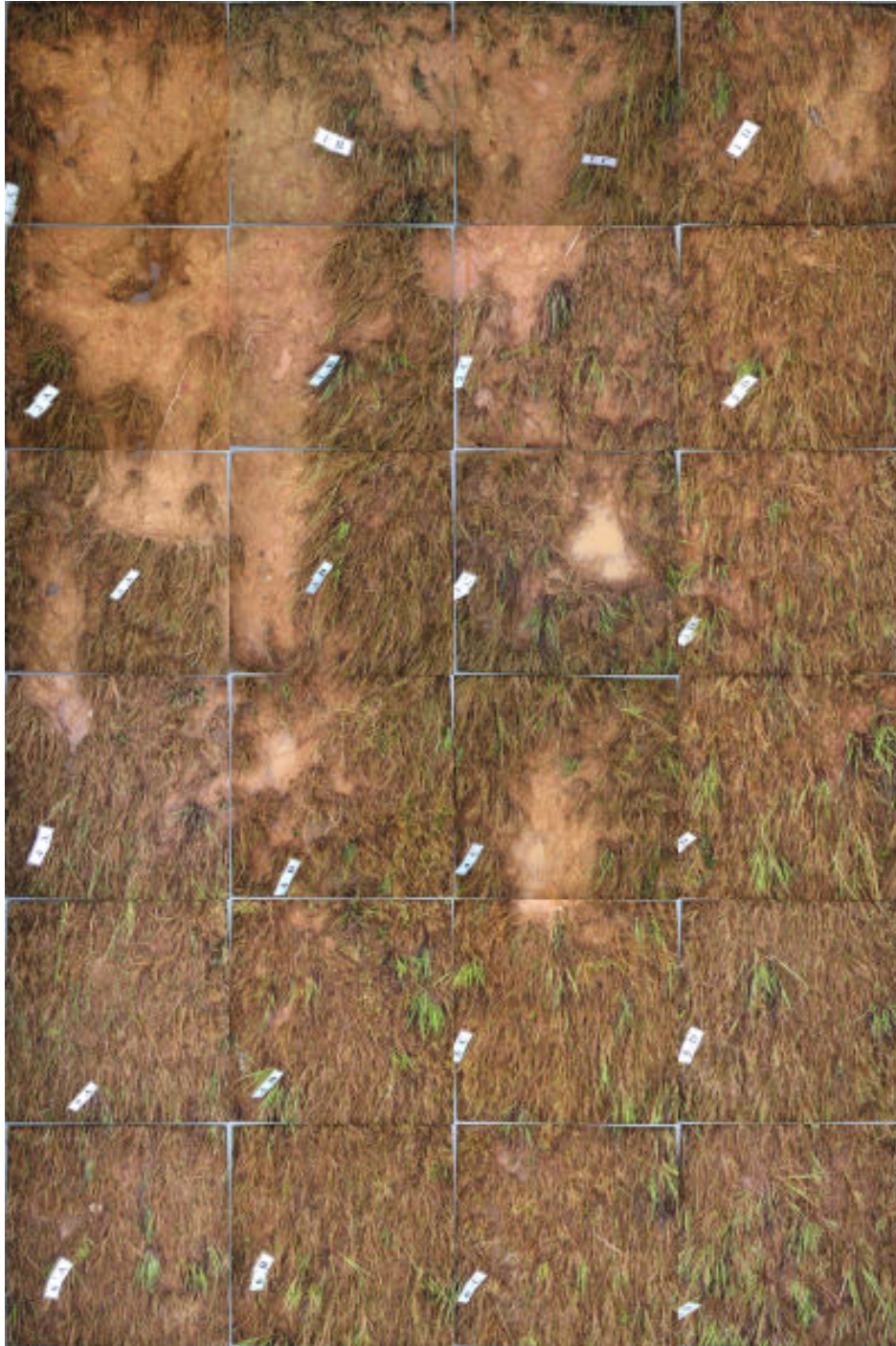
Figure B.27: 60x2 + 80x2 + 100x4 + 110x1, 1 to 6 m from the dike crest, section YB2.
