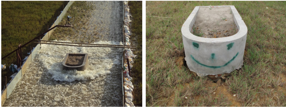
Figure 6.8: Left: flow around the round obstacle at YB1. Right: damage in front of the round obstacle.
