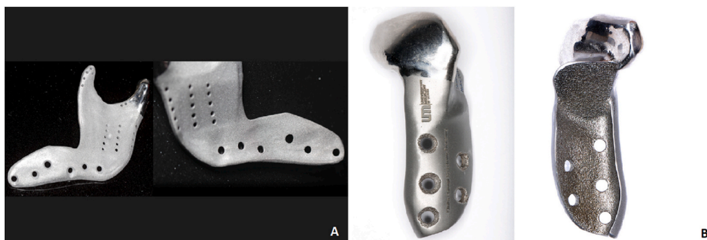
Fig. 2. Customized TMJ implants made of a titanium alloy and fabricated by using (A) CNC milling and (B) AM (DMLS) (Kozakiewicz et al., 2017).
