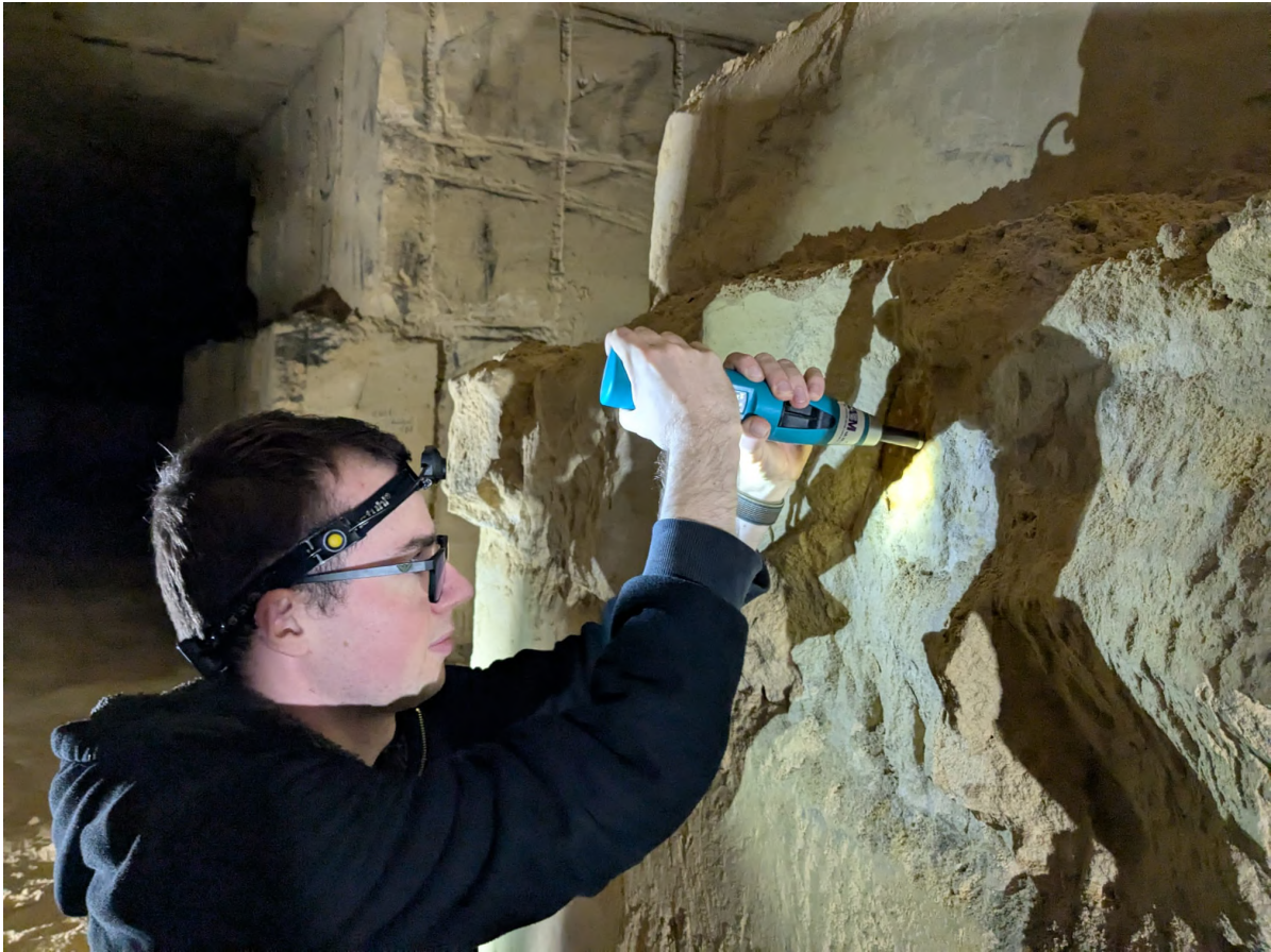
Figure F.7: The Schmidt hammer being used at ZO2-extensometer by Maxx. Own work.
