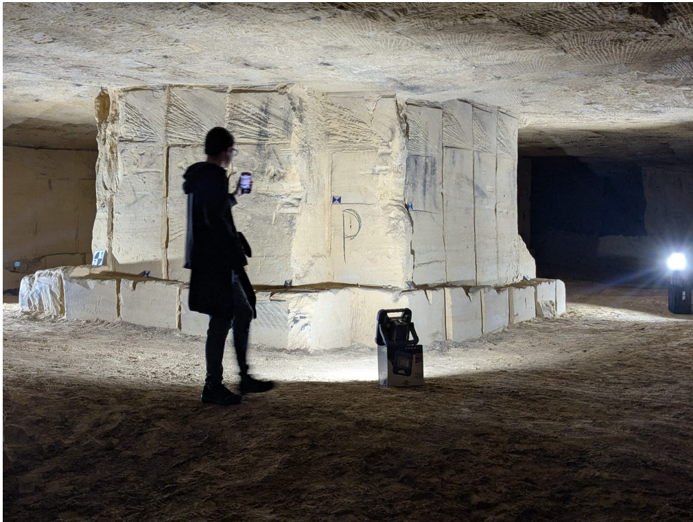
Figure 2.2: A photo taken during the scanning of one of the many pillars. All the lamps are placed at the corners of the pillar, and the iPhone is used for scanning. Photo from Roderik Lindenberg, 2025.
