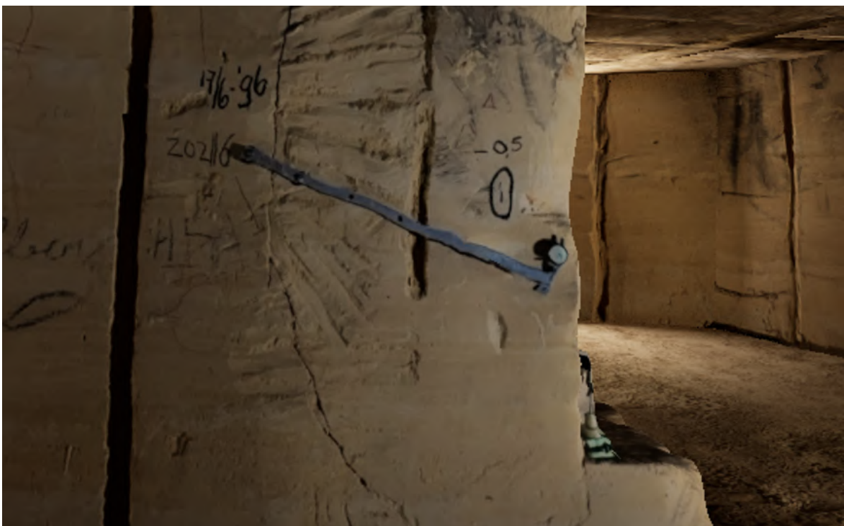
Figure F.6: The permanently installed crack-meter at ZO2-S2. Own work.
