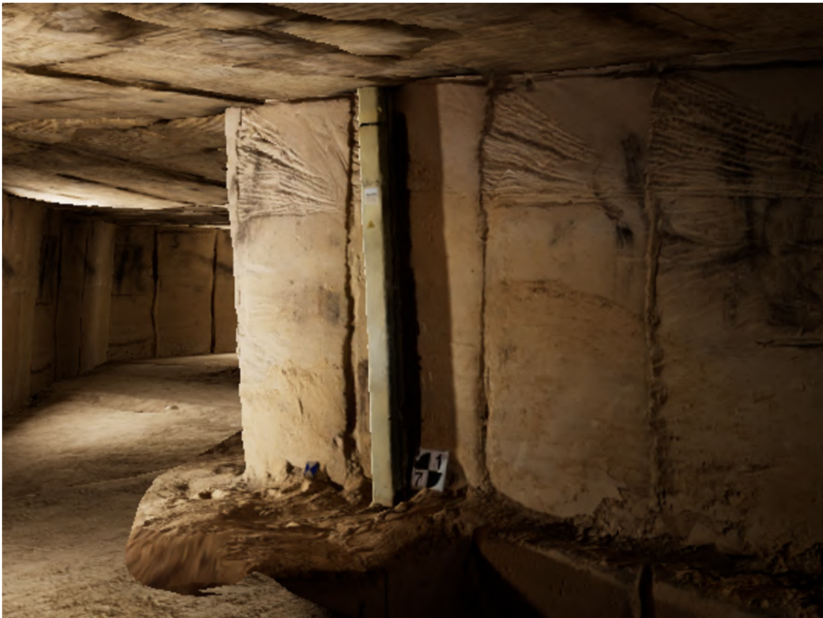
Figure F.5: The permanently installed extensometer at ZO2-S5. Own work.
