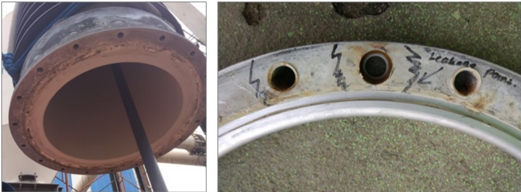
Figure 4.9 Corrosions at the inner junction between enclosures found in the case study: (left) the corrosion at the junction between the bushing termination with the GIS enclosure after 25 years of service time. The GIS is located outdoor and close to the seashore, (right) the corrosion at the inner junction between enclosures after 30 years of operation, the GIS is located outdoor at the relatively benign environment.
