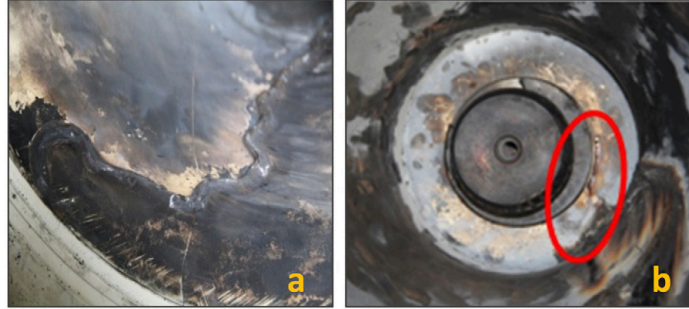
Figure 2.14. Forensic findings from Case #7: a) A carbonized track at the surface of the conic spacer, b) the melted part on the connection between the spacer and the conductor.
