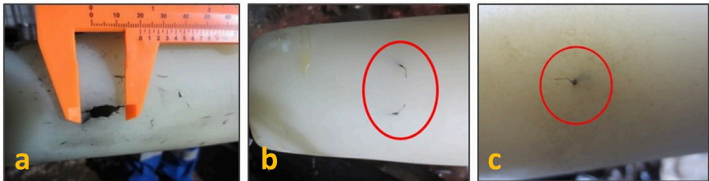
Figure 2.9 Forensic findings from Case#2: Holes found after the breakdown on the cable termination of Phase T (a), Phase S (b), and Phase R (c); on a power transformer feeder bay.
