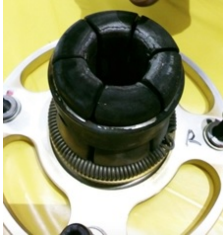
Figure 4.7 A carbonized female-main contact in one of Circuit Breaker in GIS in the case study. The measurement before opening the enclosure had shown the increase of the static contact resistance above 20% from the last result.
