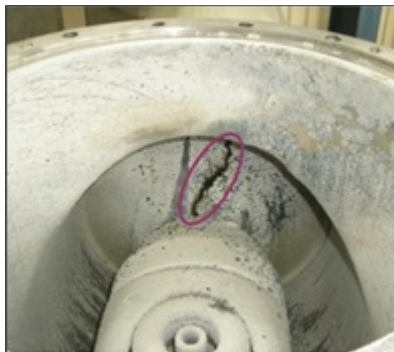
Figure 2.10 A burn mark has been discovered on the surface of the conic spacer below the ES contacts. White powders, which is a solid decomposed SF 6 by-product, was found abundantly on the affected parts.
