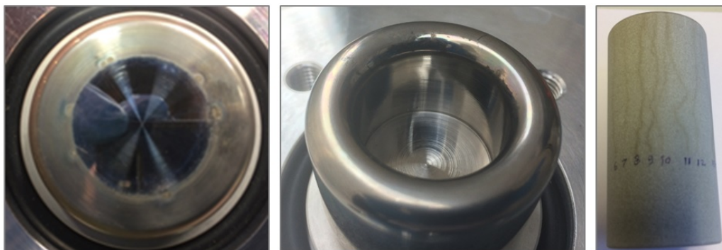
Figure 3.15 The setup after a series of tests under LI+ stress: (2 figures from the left) HV and LV electrodes of quasi-homogeneous setup, (the most right figure) an epoxy sample with flashover traces. The solid by-products, possibly the aluminium fluorides, and craters were observed in the setup after the test.
