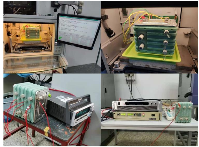
Figure 6. Electrical parameters testing of the proposed IGBT press-pack module.
