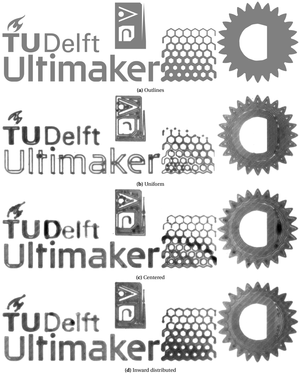
Fig. IV.16. Test shapes printed using the uniform scheme, centered scheme and the inward distributed scheme. The uniform technique produces distinct underfill areas. The centered scheme shows some defects due to inaccurate control of extreme deposition widths. The inward distributed scheme produces the least defects.
