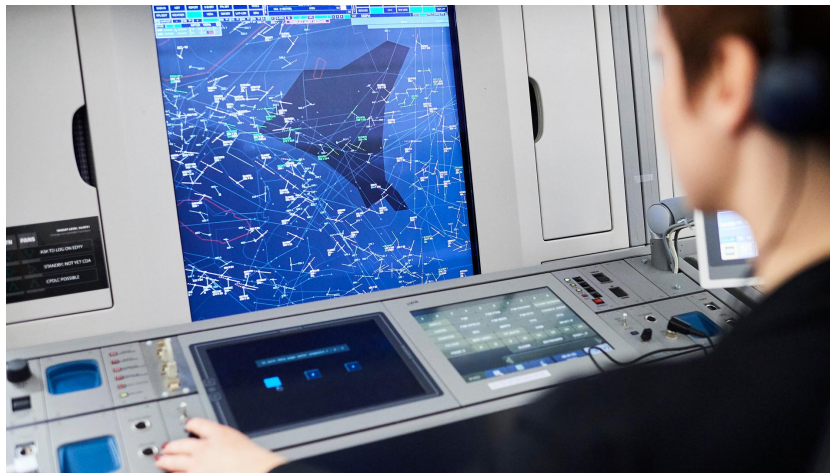
Figure A.2: MUAC radar Screen [22]
