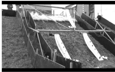
(a) Overtopping at the crest
