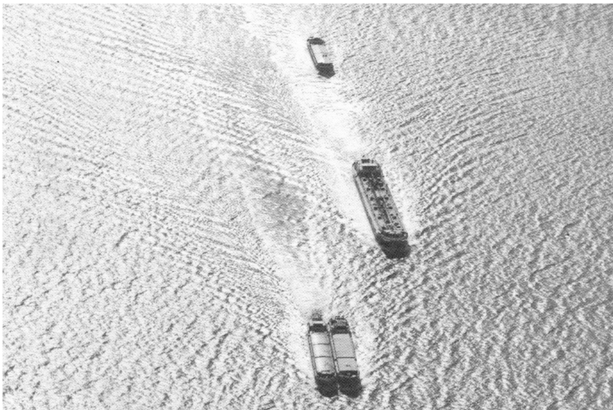
Figure 4.1: Primary, secondary and propeller jet water motion (by TU Delft – Ports and Waterways is licenced under CC BY-NC-SA 4.0).
