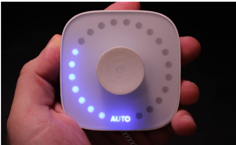
Figure 49: The dimmer in automatic mode, activated by long pressing
