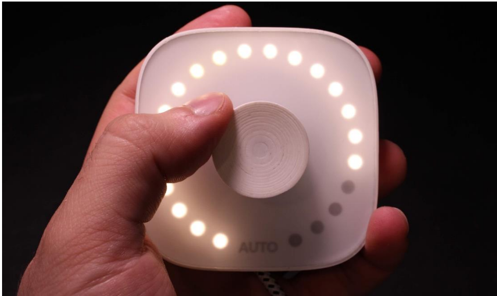
Figure 48: The dimmer in manual mode, activated by clicking or turning
