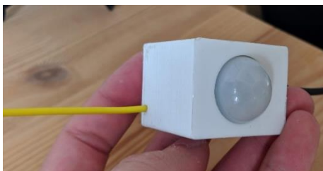
Figure 7: Homemade device with a sensor and radio control actuator.
