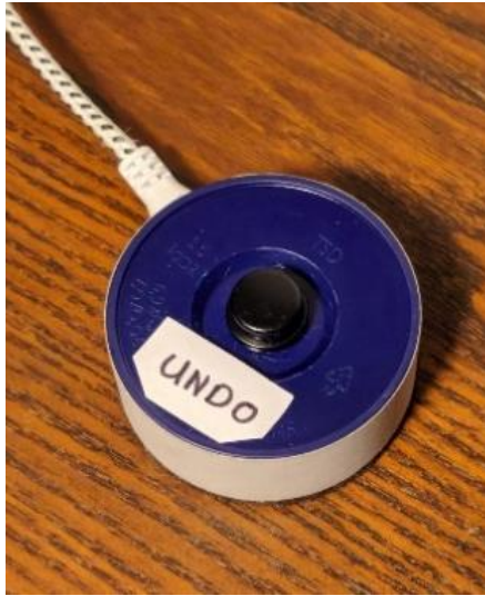
Figure 30: Scenario 1, it allowed participants to undo the latest change of the lighting. They were meant to use it when it got too dark to read.
