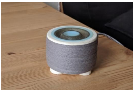
Figure 8: Homemade switch that utilizes the open MQTT protocol.
