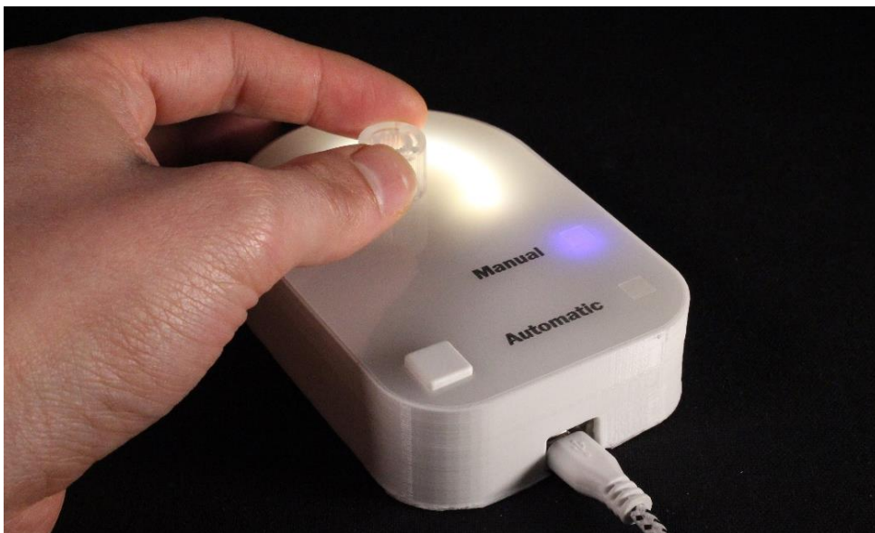
Figure 32: Scenario 3, it allowed participants to control a light and disable the automations automatically. To enable automations again, the dedicated button had to be pressed.
