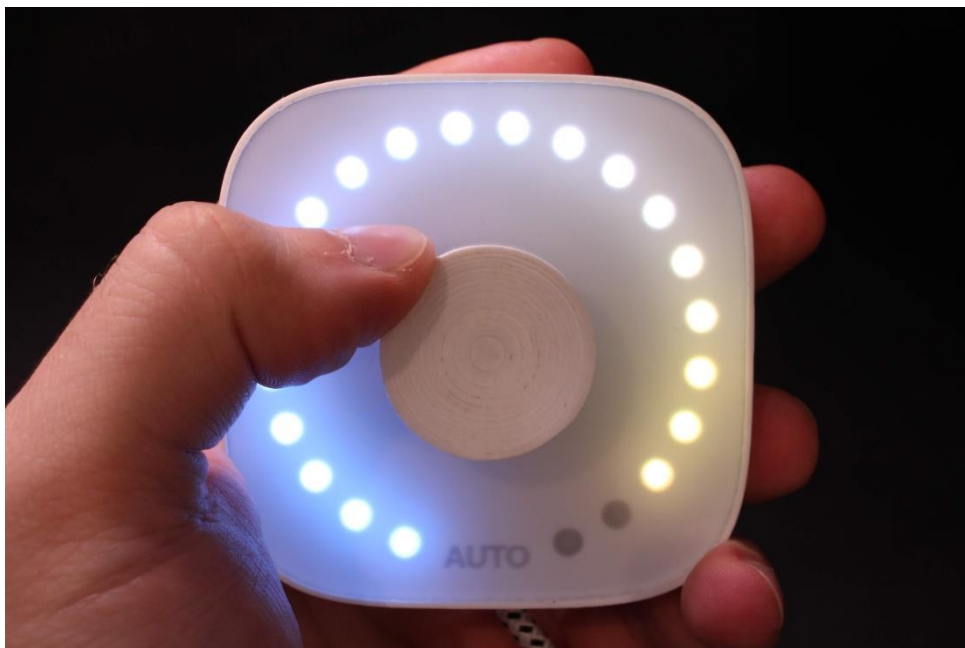
Figure 53: Custom dimmer feature used for color temperature control
