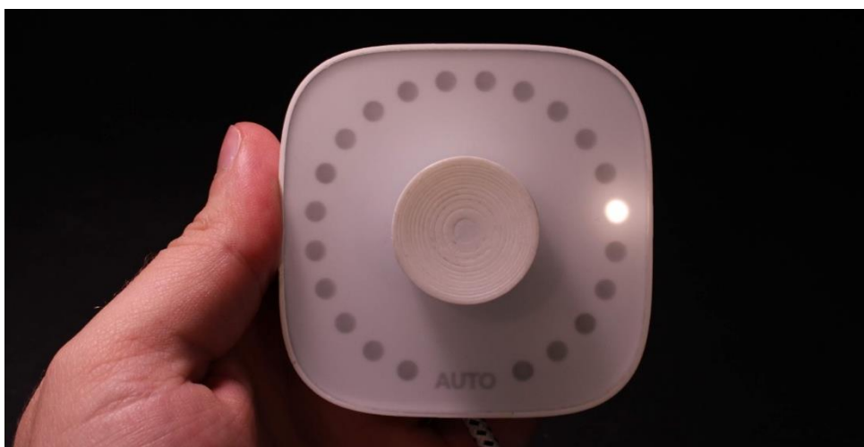
Figure 51: The dimmer when the lights are on, but haven't been changed for 10 seconds. This indicator shows the current brightness of the lights.
