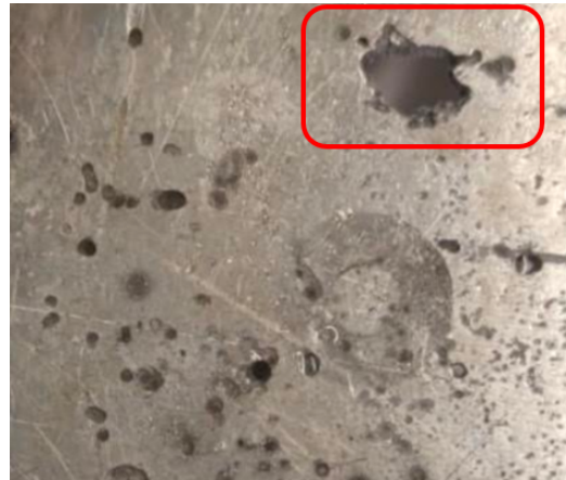
Figure 4.8: The created hole inside the workpiece encircled by the red square.
