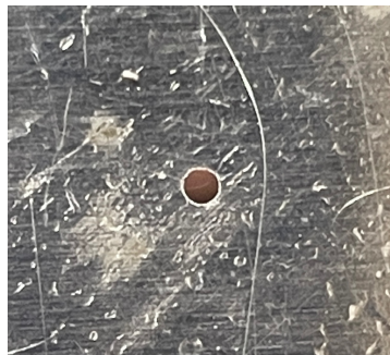
Figure 4.3: Experiment 2: The created hole inside the workpiece.
