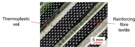
Fig. 1. Picture of an hybrid side-by-side textile based on quasi-unidirectional carbon fibres and polyetherimide veils [10]. The textile stack has a partial and staggered cutaway, unveiling the different layers of the stack.
