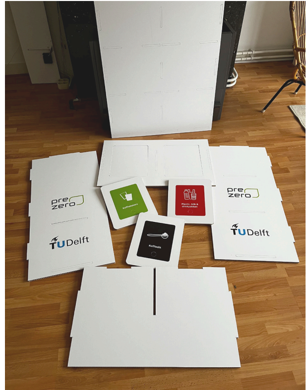
Figure 7.8 How the prototype parts as flatpack.
