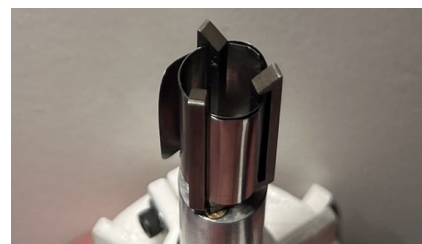
Figure 4.6: Image of blade inside device during the additional test, edge of blade extends from coil based on orientation of the blade inside the hooks due to natural tendency to expand.
