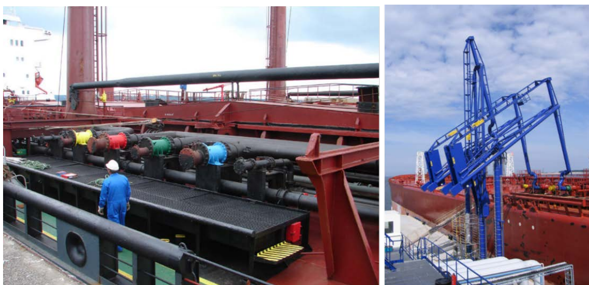
Figure 5.3: Liquid bulk (un)loading facilities; left: manifold ( Maya OBO carrier 3 by Herv Cozanet is licenced under CC BY-SA 3.0); right: (un)loading arms ( Marine Loading Arm KLEa by Ljl.kanon is licenced under CC BY-SA 3.0).
