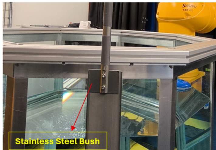
Figure A.13: Steel Bush attachment, in between the wing and the shaft slot, in order to improve the fit of the joint
