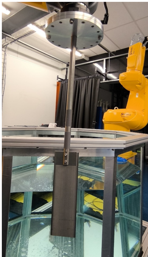
Figure 4.4: Rectangular Stainless Steel Wing Assembly attached to the Staubli Flange.
