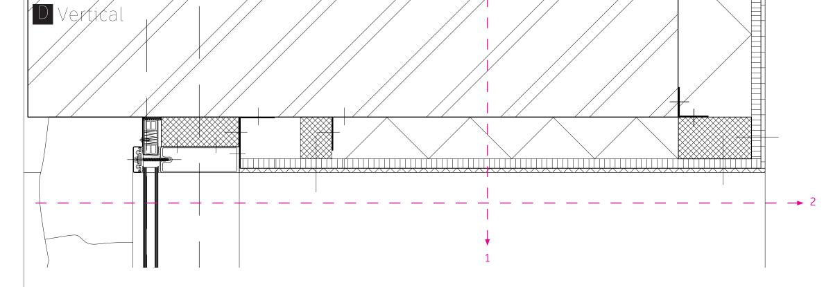
Aluminium roof profile for curtain wall roofs 250 mm + triple glass 40 mm or sandwichpanels (GRP Glass Reinforced Plasic + VIP Vacuum Insulation Panel)
