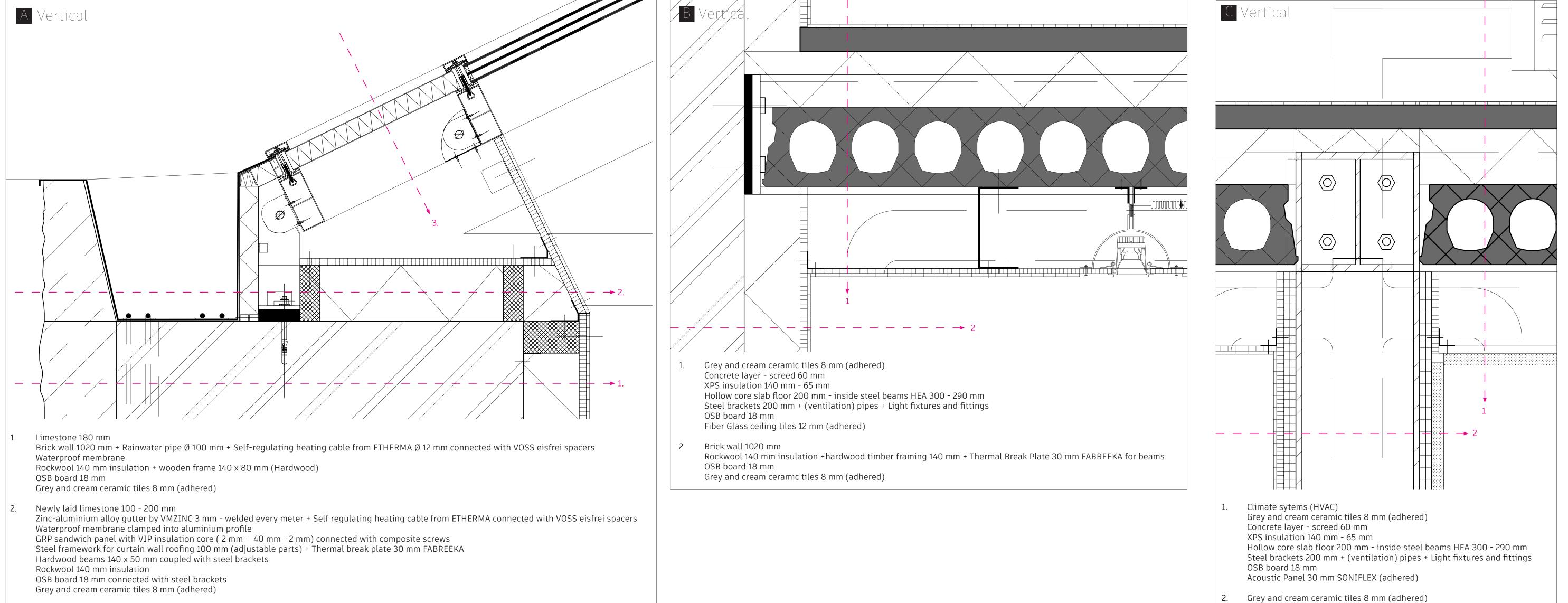
Grey and cream ceramic tiles 8 mm (adhered) OSB board 18 mm Fire resistant plasterboard 15 mm GYPROC (30 min) Fire resistant plasterboard 15 mm GYPROC (30 min) Steal beam HEA 300 290 mm + Ventilation pipes Ø 125 mm Fire resistant plasterboard 15 mm GYPROC (30 min) Fire resistant plasterboard 15 mm GYPROC (30 min) Acoustic Panel 30 mm SONIFLEX (adhered)
