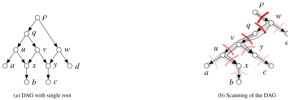
Fig. 1. A DAG with a single root (a), and a tree extension of the DAG (b), functioning as a route for the scanner lines. The tree extension is indicated by the grey edges, while the arcs of the DAG are drawn back in, following the edges of the tree extension. The scanner lines start at the leaves and move up through the tree extension, at each step becoming brighter red. The tree extension is optimal, thus the scanwidth of this DAG is 3: the maximum number of DAG arcs that are cut by one of the scanner lines. (For interpretation of the colors in the figures, the reader is referred to the web version of this article.)
