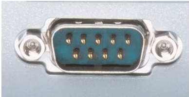
Fig. C.2: A serial port with 9 pins. Source: Ergo Canada [37]
