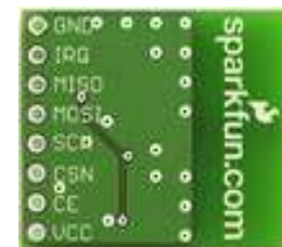
Fig. 5.5: A nRF24L01+ Transceiver. Source: Sparkfun Electronics [17]
