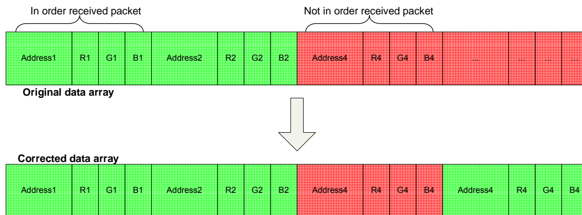
Figure 8.1: In the original data array the first two packets are received in order but packet number three is missing which will dislocate all the other packets and ruins the image. In the second data array the addresses are rearranged in the correct order filling up the not received packets with the packet next to it.
