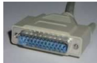
Fig. C.1: A parallel port with 25 pins. Source: Wikipedia [35]
