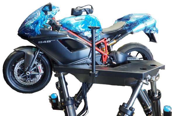
Figure 1.1: Picture of the Cruden motorcycle simulator. The simulator consists of a Ducati 848 Evo motorcycle mock up mounted on a Stewart platform.
