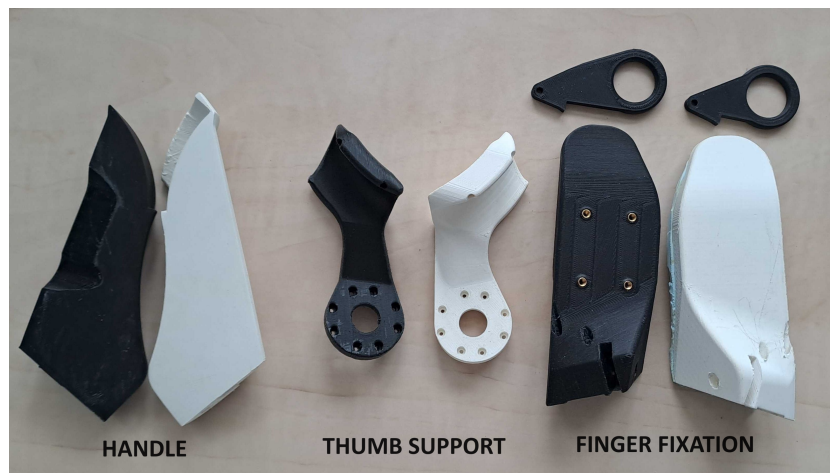
Figure C.2: Modified parts (black) next to the original counterparts (white) of the hand rehabilitation robot designed by Rätz et al. [5, 4] to improve the integration of the tactile interface into the robot.
