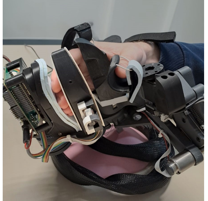
Fig. 1. Tactile interface device developed in the present study, assembled into the hand rehabilitation robot by Rätz et al. [1]. The device, in contact with the fingerpads, provides force-controlled skin stretch stimulation, which allows for accurate rendering of tangential forces, like the weight or the friction forces, when interacting with a virtual tangible object.
