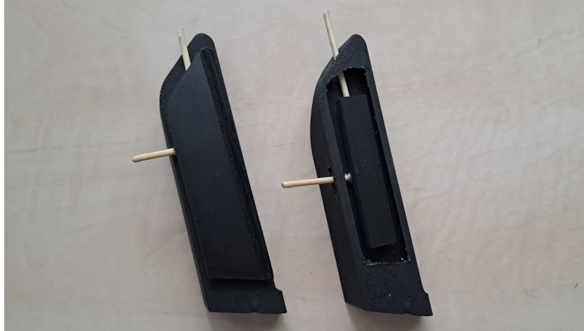
Figure A.1: Mock-ups used for comparing the sensation provided by a fully actuated platform and a multidigit tactor-like design with a frame for grounding the outer area of the finger pads.
