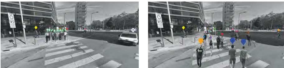
Figure 3. Moodility illustration: if enough people want to cross the light turns green and pedestrians take precedence over cars - [CC-BY-NC 4.0 C. Gauchet Dumortier | C. Derue | E. Braconnier | N. Brooks]
