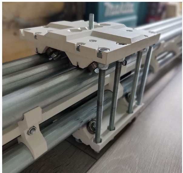
Figure 53: Y-Axis Carriage mounted to conduits
