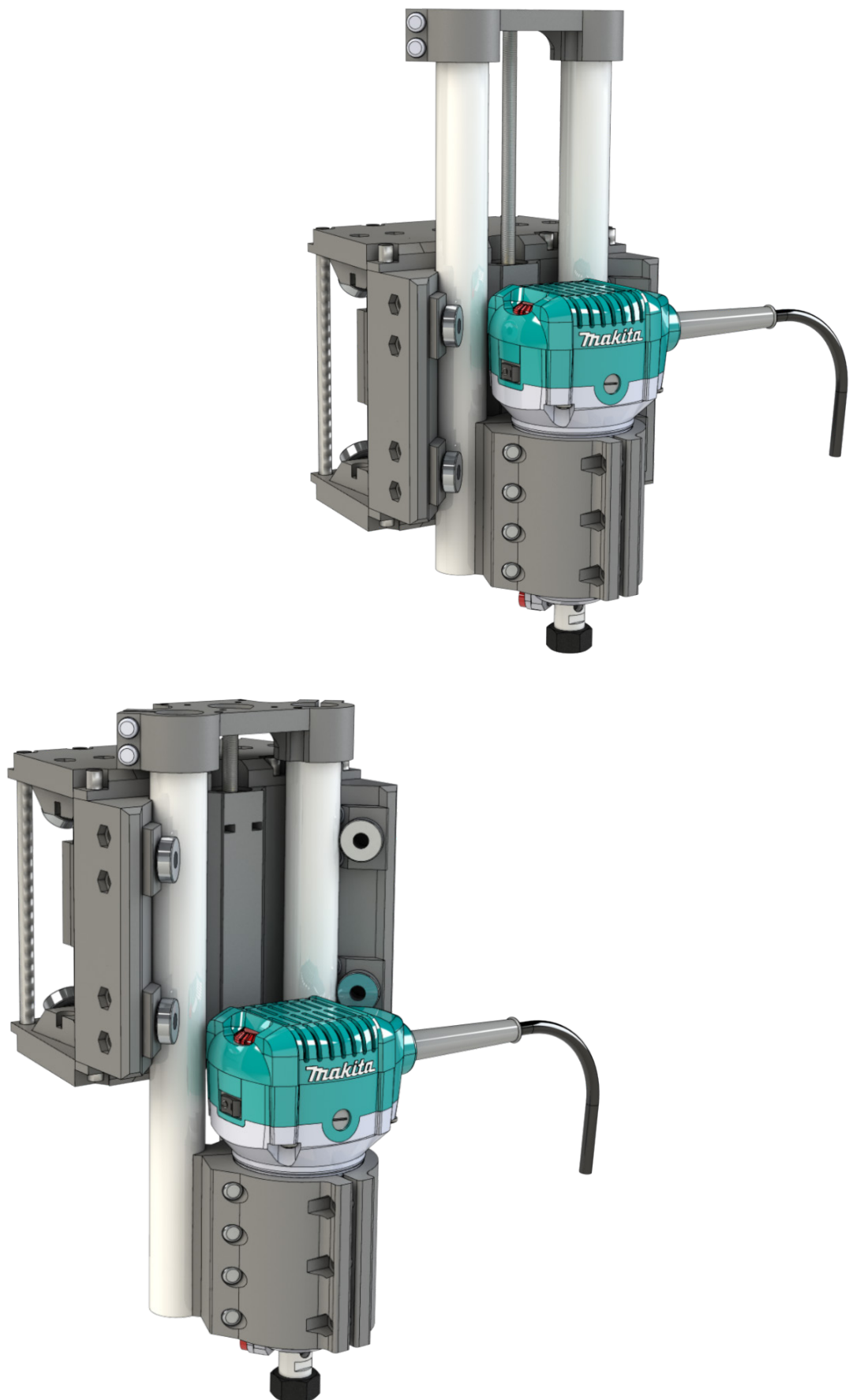
Figure 63: Vertical linear motion of Z-Axis
