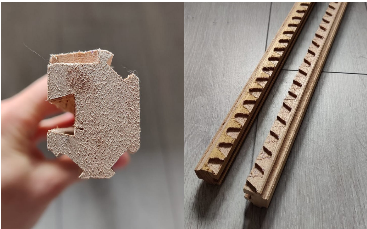
Figure 37: Manufactured Meranti Profiles
