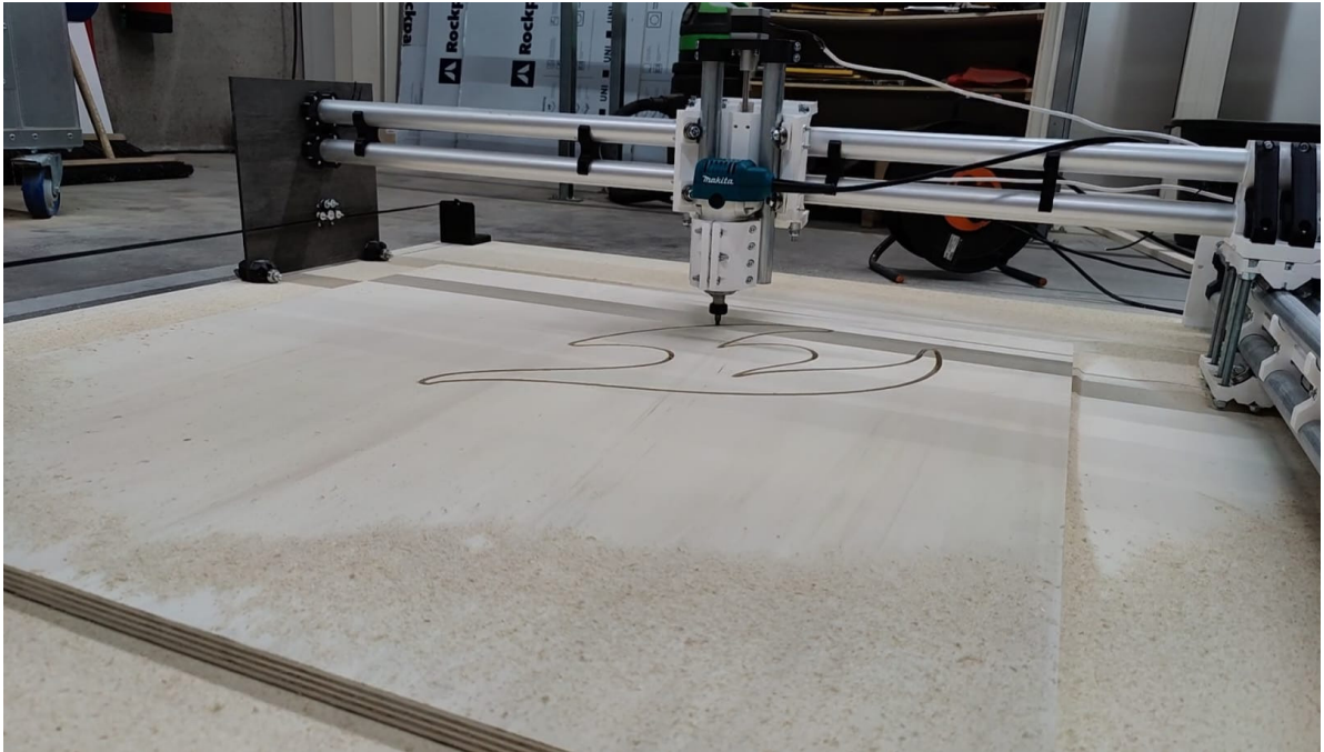
Figure 84: Delft University of Technology logo being machined from 18mm thick poplar
