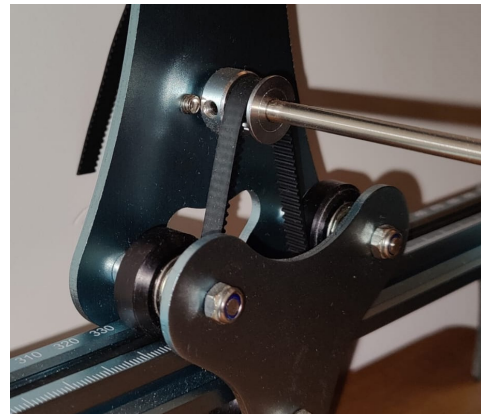
Figure 49: Motor holder & Idler pulley orientation on a laser engraver
