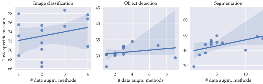
Figure 2.5: Results of selected challenges plotted against the number of data augmentations used in each entry. Each challenge shows a correlation where larger number of augmentation methods correlates with better performance. Each dot represents an entry in the final rankings. Lines represent regression model fits performed by Seaborn [30]. We exclude the action recognition and re-identification challenges as they have too little entries to analyze.
