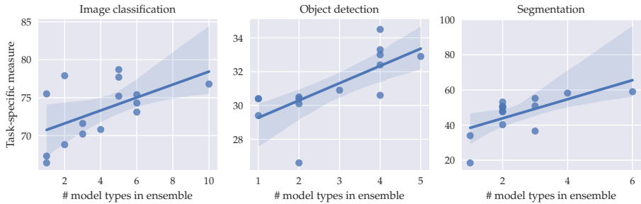
Figure 2.4: Results of selected challenges plotted against the number of distinct backbone types used in each entry. Each challenge shows a correlation where larger ensemble size correlates with better performance. Each dot represents an entry in the final rankings. Lines represent regression model fits performed by Seaborn [30]. We exclude the action recognition and re-identification challenges as they have too little entries to analyze.
