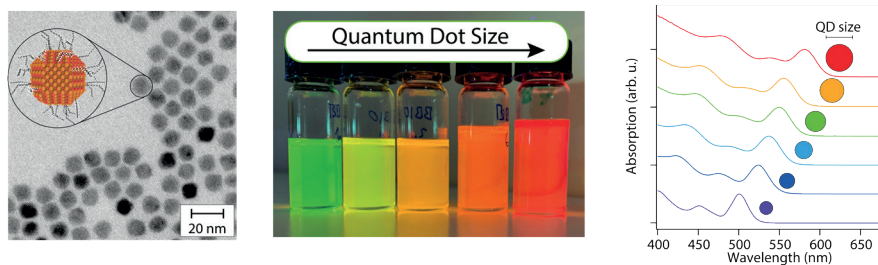
Figure 1.2. a , TEM micrograph of a QD sample. The inset show a 3D representation of a single QDs capped with oleate ligands. b , Picture showing the effect of QD size on the color of QD solutions, due to the shift in the wavelength of the first absorption feature. c , Absorption spectra of different sizes of QDs.
