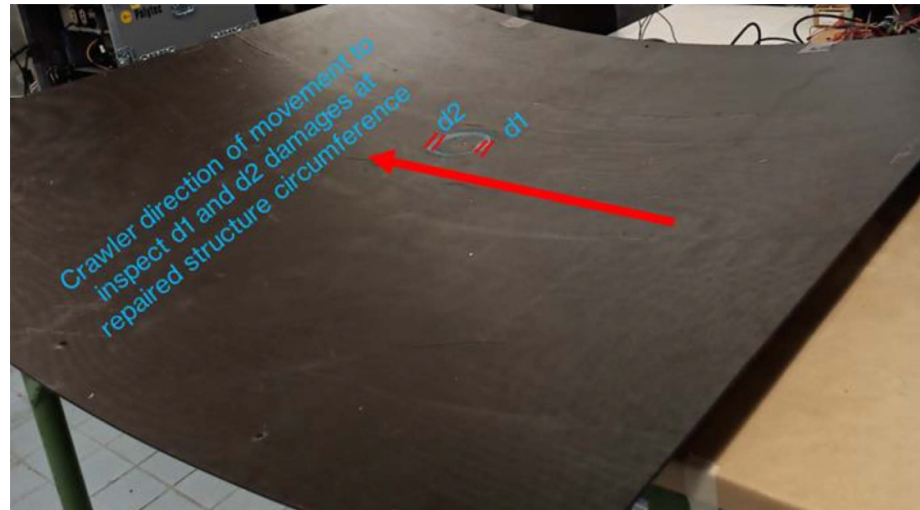
Figure 4. Diagram of the big curve composite structure with repaired damage and inspection line d1 and d2.
