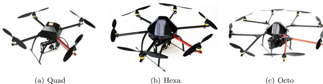
Figure A.1: Different multirotor configurations [2][3][4]
