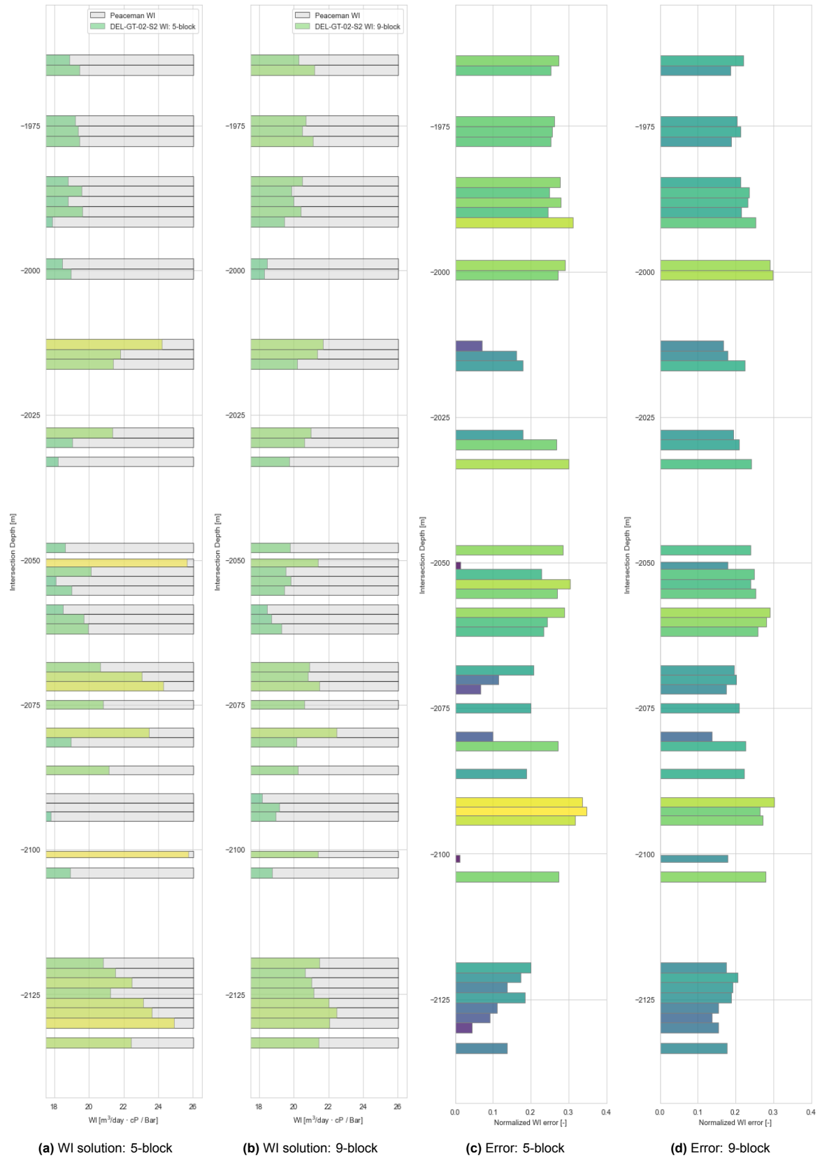
Figure 5.6: Computed well indices and normalized well index errors for the DEL-GT-02-S2 well employing both a 5-block and 9-block model.
