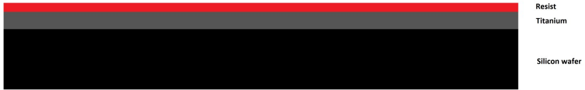
Figure 7: Configuration of the substrate, with a resist applied before patterning. On the bottom the silicon wafer, on top of the wafer 200 nm evaporated titanium and on top the resist.
