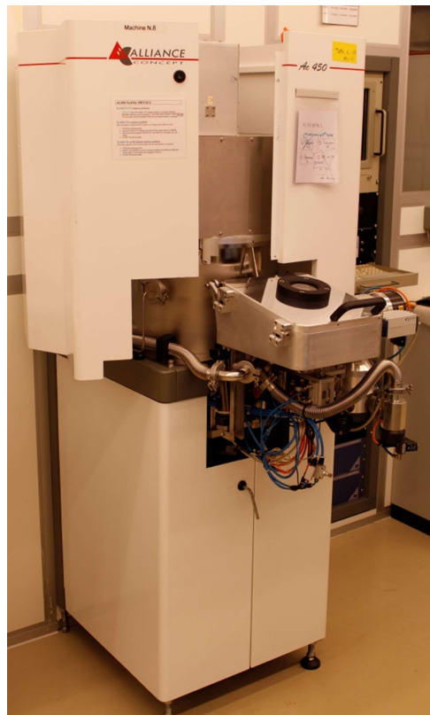
Figure 11: Ion milling equipment used (Alliance concept Ac450). On the front the load lock of the machine can be seen.
