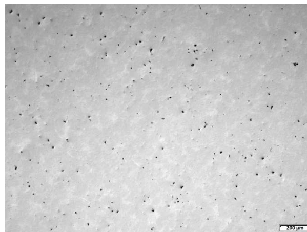
Figure 16: Optical microscope image of the result of automatic polishing, the scale bar is 200 µm. The surface texture can be seen, some voids in the material and some micro roughness can be seen on the surface.
