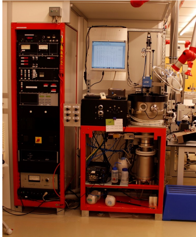
Figure 10: RIE equipment used (Leybold Hereaus). On the right the control system can be seen, and on the left the chamber (cylindrical) can be seen.
