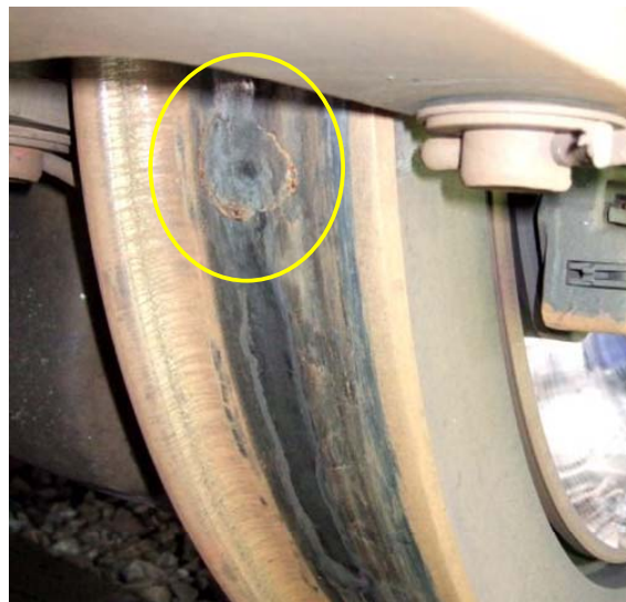
Fig. 5.1 Illustration of a wheel flat formed by wheel-rail slip in the contact
