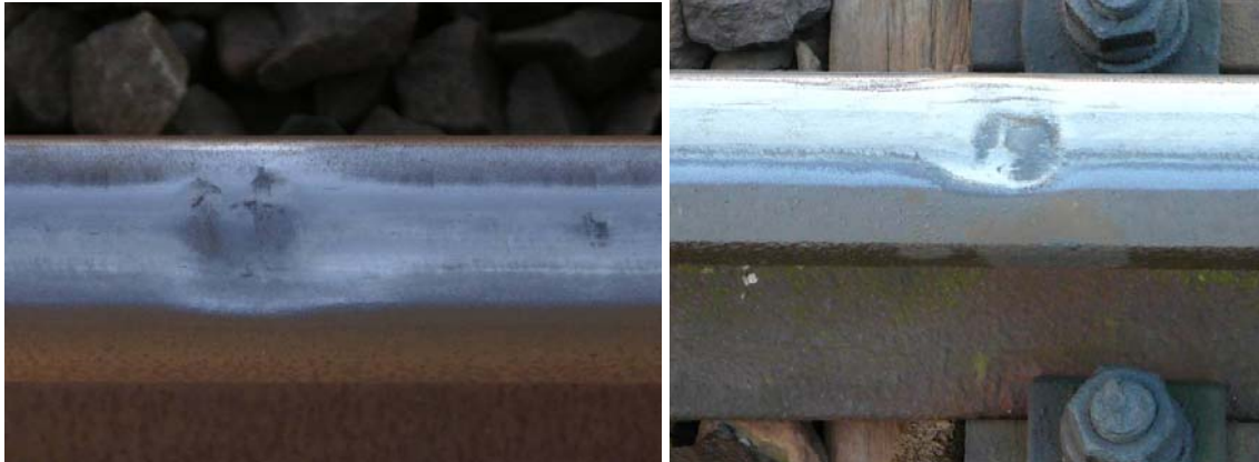
Fig. 1.9 Squats on the rail surface in the contact band
