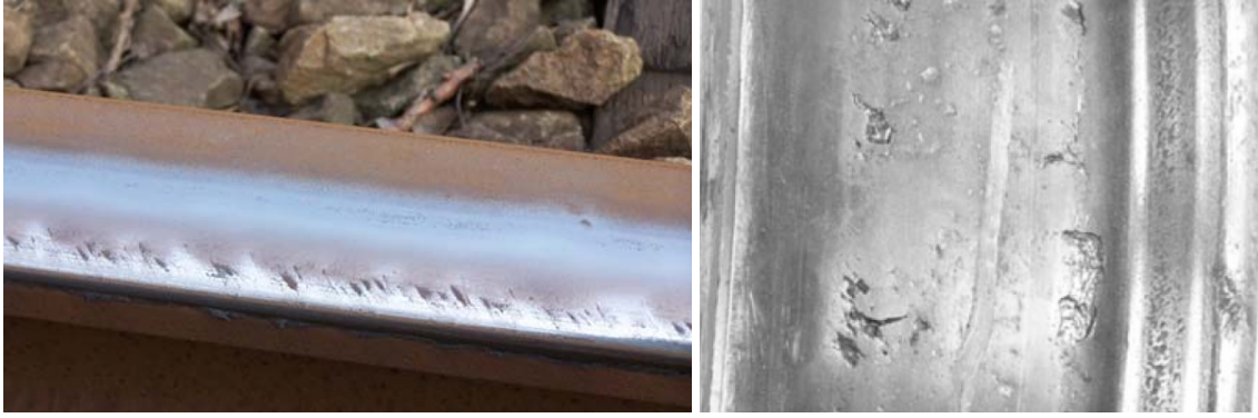
Fig. 1.8 Head checks (left) and RCF damage on a wheel tread (right; from [1.27])
