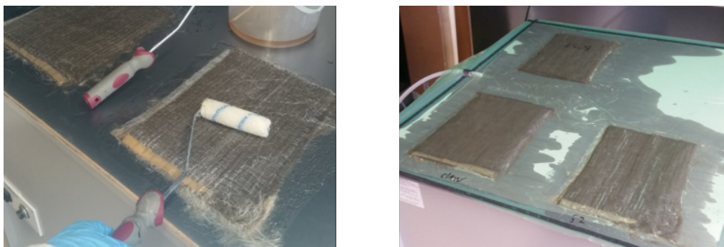
Figure 3.9: (a) Hand layup method, (b) Sealing tape for vacuum application while curing
