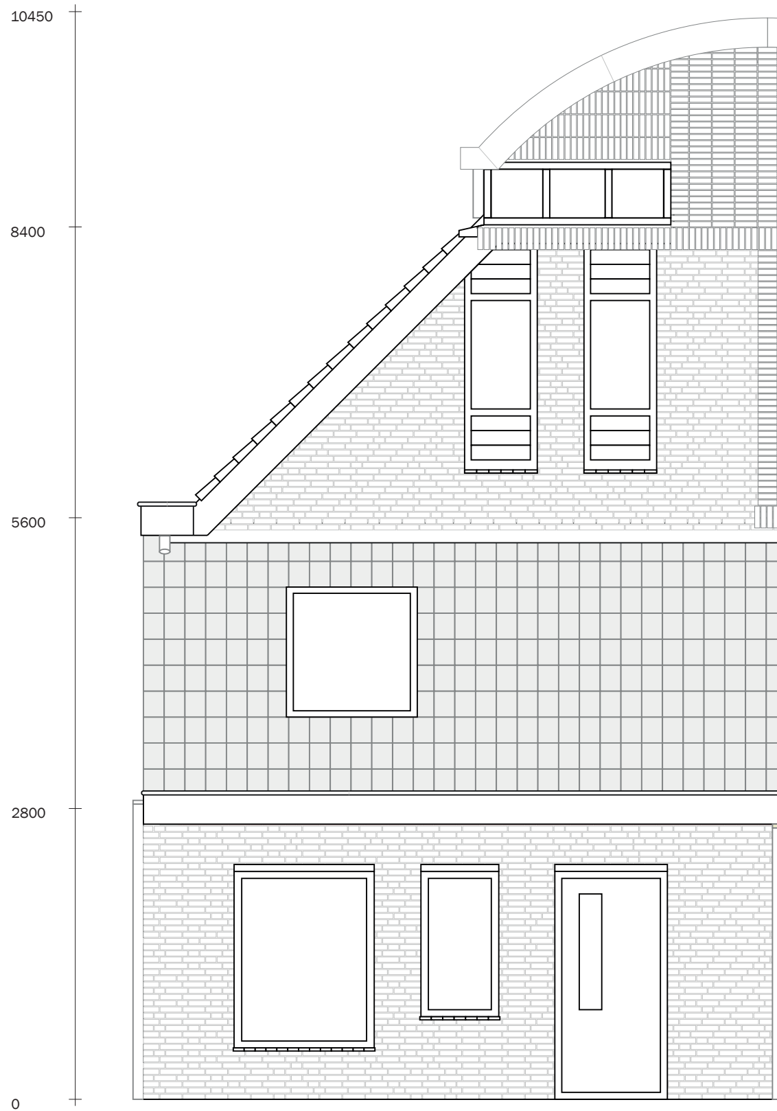
Fig. 69 Facade design 1:50, left: private that does not participate in full renovation, right: Ymere home with home split and full renovation
