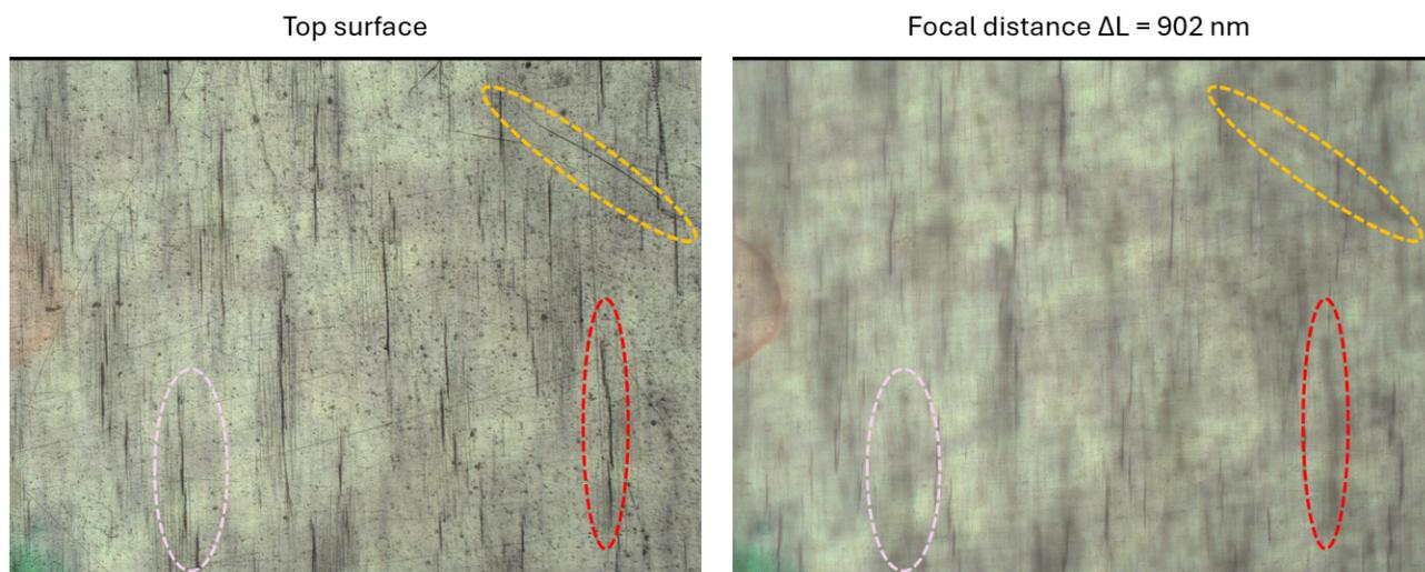
Figure 6.8: Microscope image comparison between the top surface and the underlying layer.
