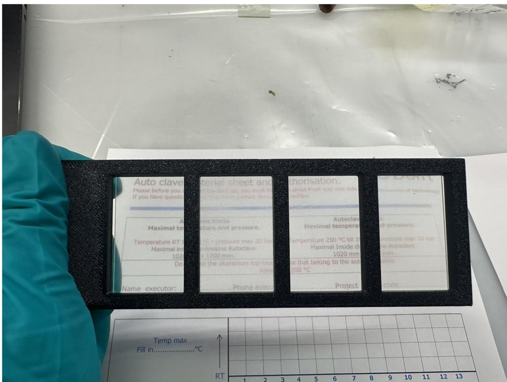
Figure 5.10: Transparency of the TGFRP samples at a distance from a sheet of text. From left to right: 0% MMA, 0.5% MMA, 1.0% MMA, 2.5% MMA.
