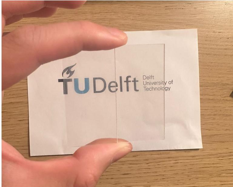
Figure 5.19: Pure resin sample (left) vs post-cured resin sample (right).
