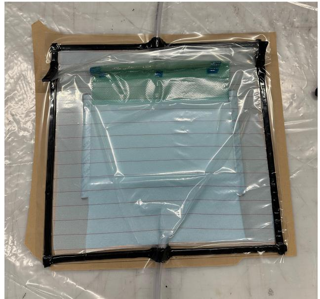
(b) Final assembly before the leakage test.
