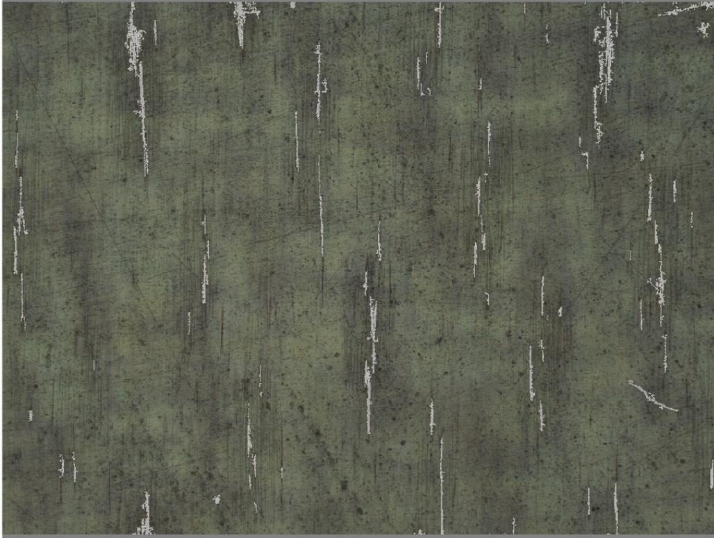
Figure 6.11: Image processing for crack detection: cleaned binary image overlaid on the original image.
