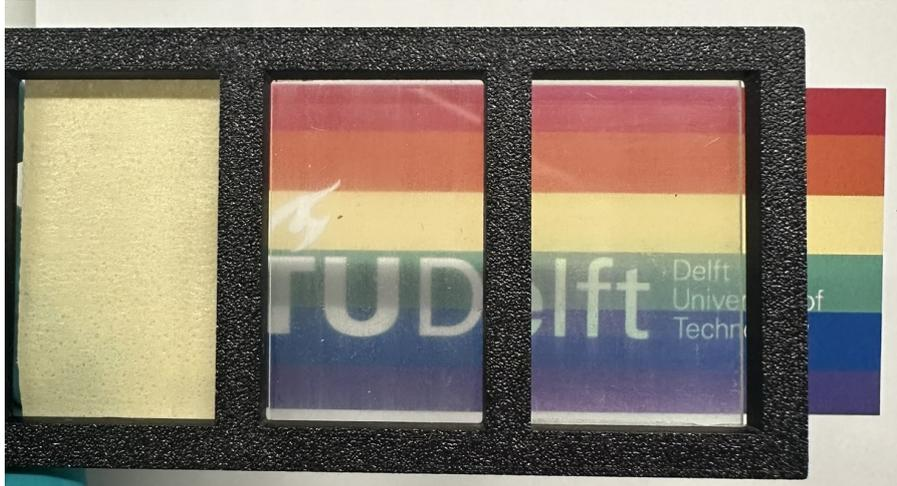
Figure 5.5: Pure resin sample (left) vs. TGFRP sample (right) at a distance from the TU Delft logo.
