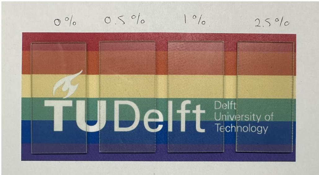
Figure 5.9: Transparency of the TGFRP samples directly on top of the TU Delft Logo. From left to right: 0% MMA, 0.5% MMA, 1.0% MMA, 2.5% MMA.
