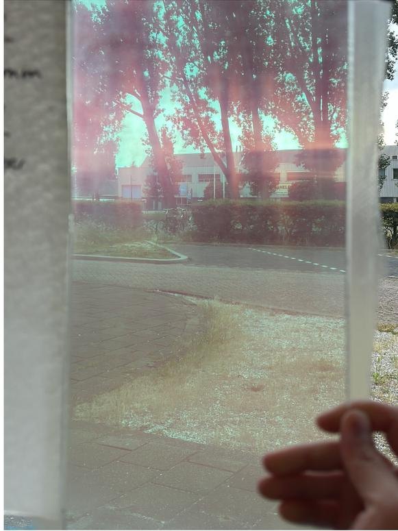
Figure 5.2: TGFRP panel produced using the modified VIP with resin from R&G.
