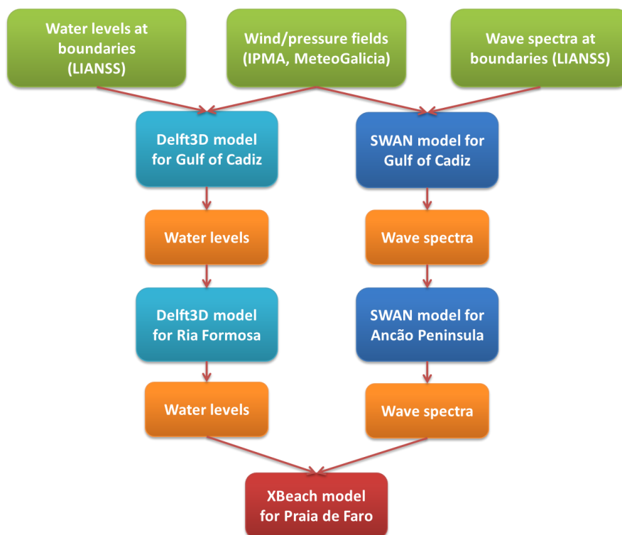
Figure 4-1 Scheme of the model train for Praia de Faro.
