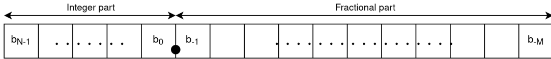
(b) Unsigned representation with an M bit fractional part and an N bit integer part.
