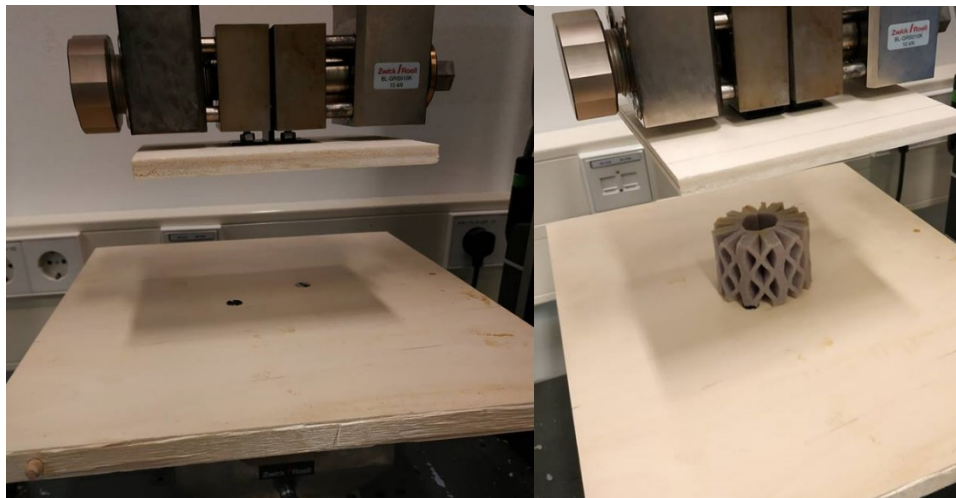
Figure X | Zwick Z010 material testing machine is initialized and calibrated using textXpert II software.
