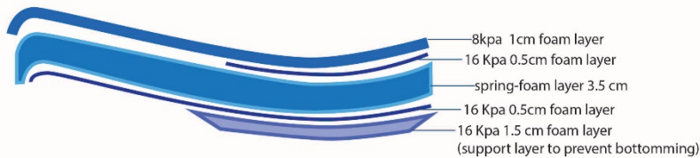
Figure 2: Side view of seat-foam showing layer composition
